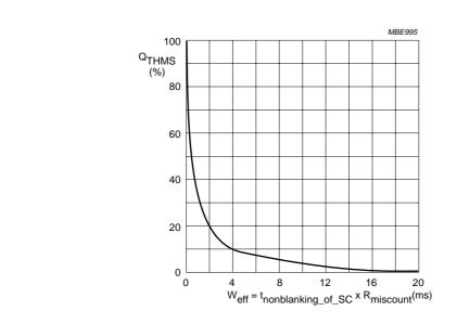
$R_{miscount}$  = ratio of effective histogram measuring time and active video in one field defined by the non-blanking periods of the sandcastle signal in one field.
